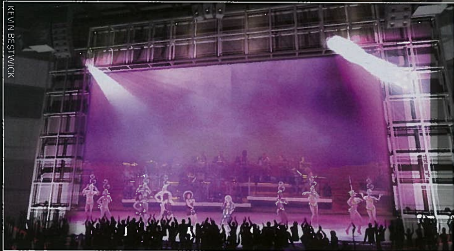
Sixty percent of the stage is covered with acoustic liner and/or panels to help with the high frequencies.
